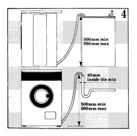
Finally, make sure that with the machine in position, the drain hose is not obstructed, blocked or bent so sharply that water cannot flow freely. The electrical connections
